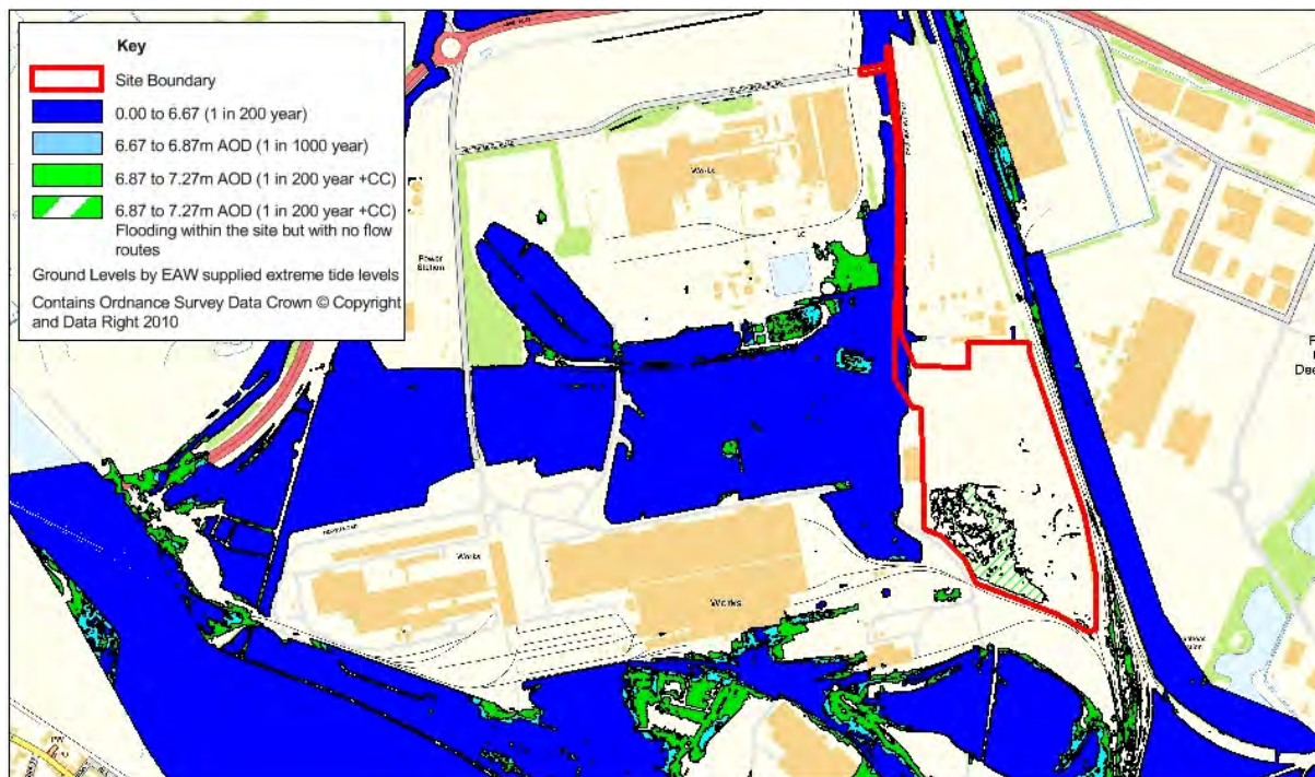
Figure 4: Contour mapping of the modelled flood levels and the ground model
