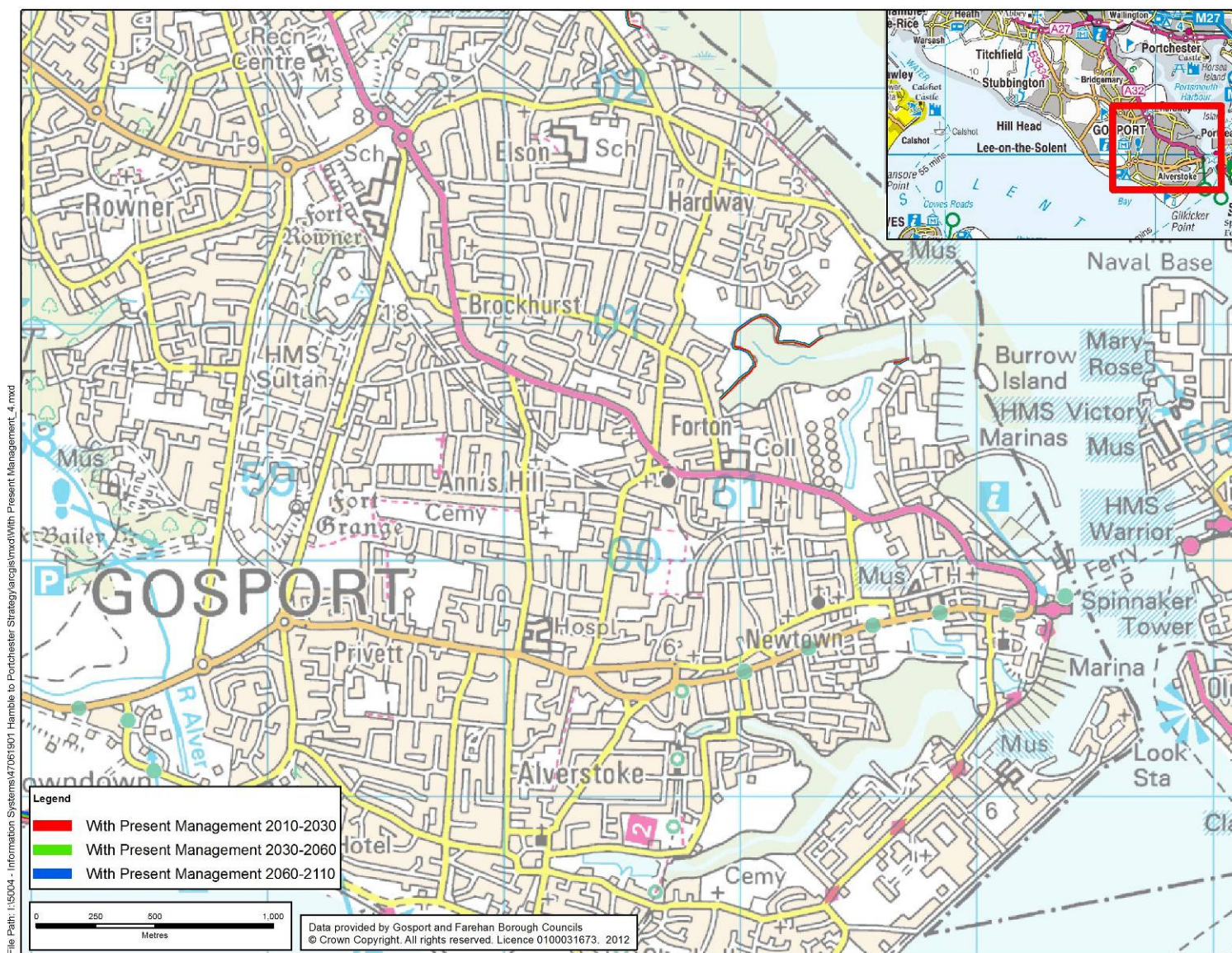
Figure 10d. With Present Management erosion lines Haslar Wall to Hardway. Source: North Solent SMP2, 2010.
