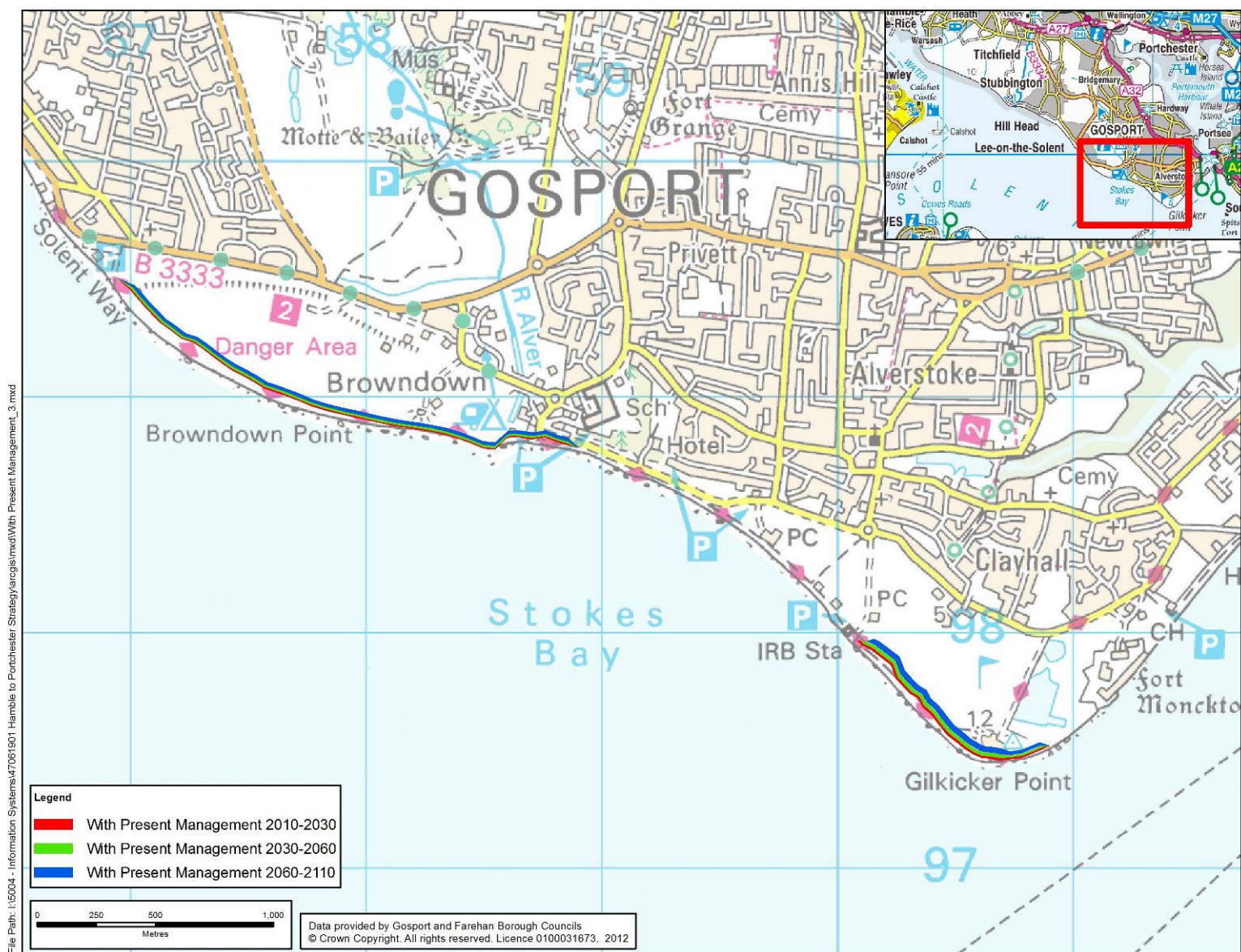
Figure 10c. With Present Management erosion lines Browdown Ranges to Haslar Wall. Source: North Solent SMP2, 2010.
